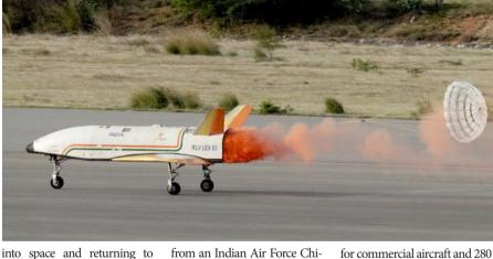
Earth like a space plane. The success of RLV LEX-03 follows the achievements of the previous missions, LEX-01 and LEX-02, and demonstrated the autonomous landing capability of the RLV under more challenging conditions. The recent test involved a cross-range of 500 meters, compared to 150 meters for LEX-02, and more
